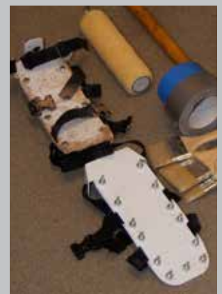
Spike slip-ons are a must for walking over epoxy without marring it.
